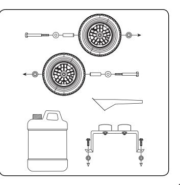
Your generator requires some assembly. This unit ships from our factory without oil. It must be properly serviced with fuel and oil before operation.
