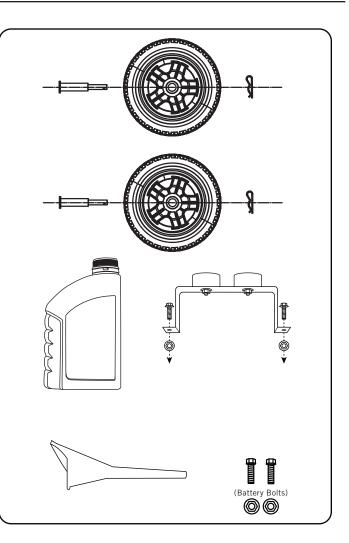
Your generator requires some assembly. This unit ships from our factory without oil and fuel. It must be properly serviced with fuel and oil before operation.
