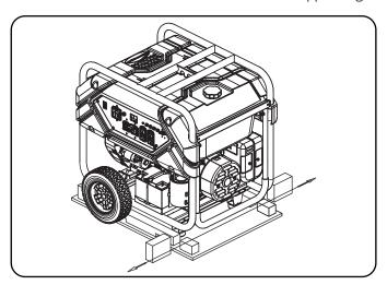
9. Slide the unit forward until the wheels touch the ground. Then raise handle to pull the unit out from the wood pallet.
