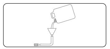
5. Pour the antifreeze into the funnel, then pull on the engine recoil starter to create suction in the pump housing. Pull the recoil several times until antifreeze comes out of the pump outlet. DO NOT START THE ENGINE WHEN DO THIS. Only pull the recoil cord if the fuel valve and engine switch are in the OFF position.
