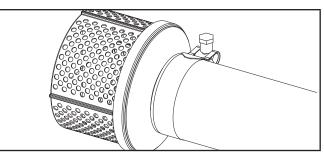
21. Tighten the clamp to 7.4 $\pm$ 1.5 lbf-ft (10 $\pm$ 2 Nm) with a 10mm wrench. If you do not have a torque wrench, hand tight then  $\frac{1}{4}$  turn past full tight.
