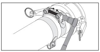
11. Once tightened, visually confirm the hose is raised on the ribs. This indicates you have it tight.
