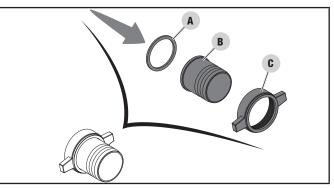
2. Thread the assembled connector to the outlet fitting (top of pump).
