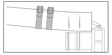
7. Insert the cam lock coupler in the green rigid suction hose until properly seated.
