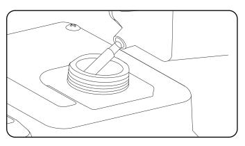
6. Screw on the fuel cap and wipe away any spilled fuel.
