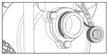
14. Thread the fitting over the tape and hand tighten.
