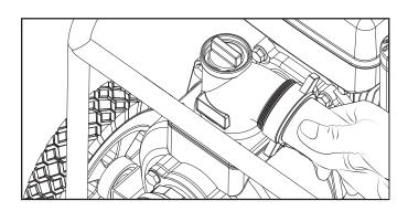
Slide the hose clamp in place about midway on the outlet hose adapter as shown. Tighten to 7.4±1.5 lbf-ft (10±2 Nm) with a 10mm wrench. The hose clamp should be placed behind the outlet adapter barbs on the smooth part of the adapter.
