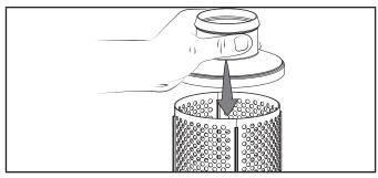
19. Place the clamp marked 54-57 on the other end of the green hose. Attach the strainer to the green suction hose.
