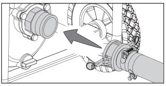
16. Lock in place with the cam levers.
