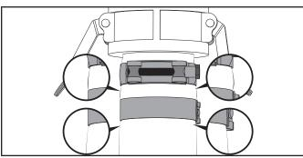
12. Test connection is tight by twisting coupler in the hose to make sure it doesn't turn. If coupling turns, then tighten clamps further until coupling won't turn.
