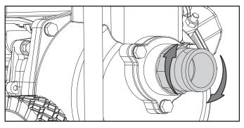
15. Attach the cam lock coupler to the fitting.
