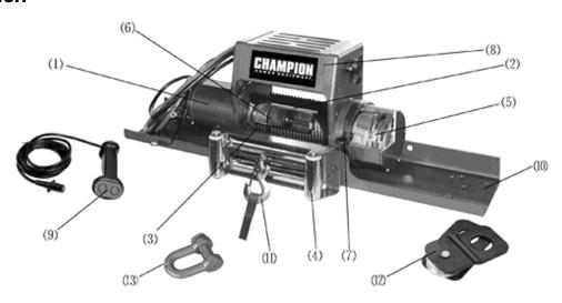
**Motor (1)**: 2.2HP motor requires a 650CCA 12 volt battery and provides power to the planetary gear mechanism.
