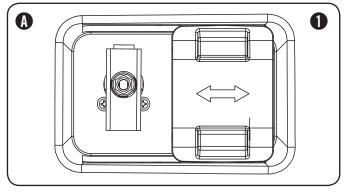
Once a fuel source has been selected, the user must turn the fuel valve to the vertical position to open the fuel valve. (1)
