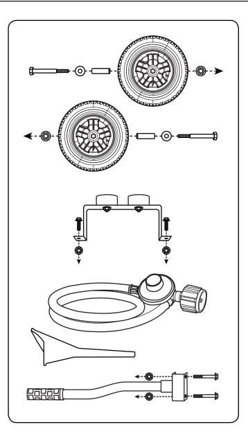
Your generator requires some assembly. This unit ships from our factory without oil. It must be properly serviced with fuel and oil before operation.
