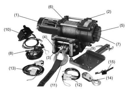
**Motor (1)**: 1.2 HP 12V DC motor provides power to the planetary gear mechanism. **Winch Drum (2)**: The winch drum is the cylinder on which the wire rope is stored. It can feed or wind the rope depending on the remote winch switch.
