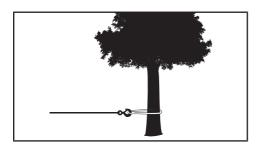
Your winch is equipped with a roller fairlead to help guide the cable/rope and to reduce binding on short side pulls. Do not winch from an acute angle as the cable/rope will pile up on one side of the drum causing damage to cable/rope and the winch.
