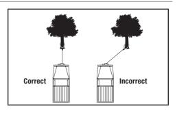
Short pulls from an angle can be used to straighten the vehicle. Long pulls should be done with the cable/rope at a 90° angle to the winch/vehicle. When pulling a heavy load, place a blanket or jacket over the cable/rope 5-6°  $(1.5-1.8\ m)$  from the hook. In the event of a broken cable/rope it will dampen the snap back.
