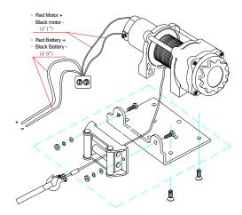
8. Connect the red (positive) lead of the switch assembly to the positive (+) terminal of the motor. Connect the black (negative) lead of the switch assembly to the negative (-) terminal of the motor.
