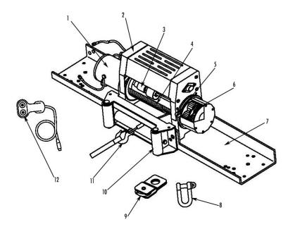
(1) Motor - 3.6 Hp 12V DC motor provides power to the planetary gear mechanism.
