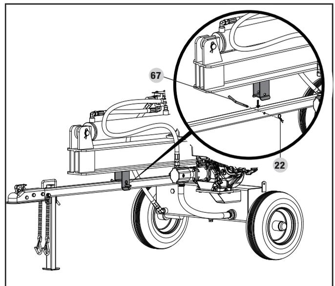
2. Standing alongside the hydraulic ram, (opposite side from the engine) firmly grasp the handle on the beam and lift upward while pushing the beam back until upright. (Caution, beam is heavy.)
