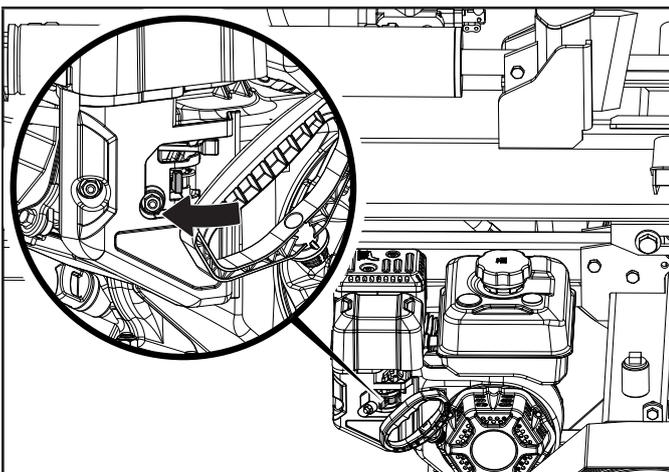
2. Let the engine run until fuel starvation has stopped the engine. This usually takes a few minutes.
