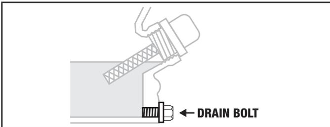
2. Allow the oil to drain completely into an appropriate container.
