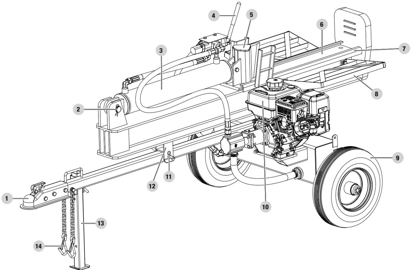
1. **2 in. (5.1 cm) Ball Coupler** – For towing the log splitter behind your vehicle.
