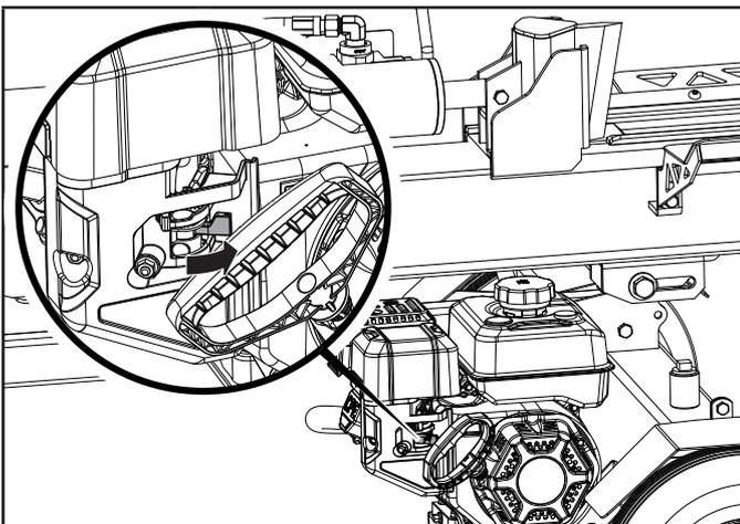
3. Move the choke lever to the "CHOKE" position.
