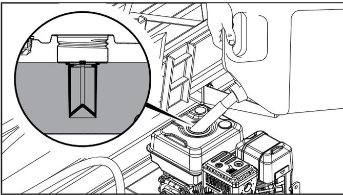
5. The approximate fuel level is shown on the fuel gauge on top of the fuel tank.
