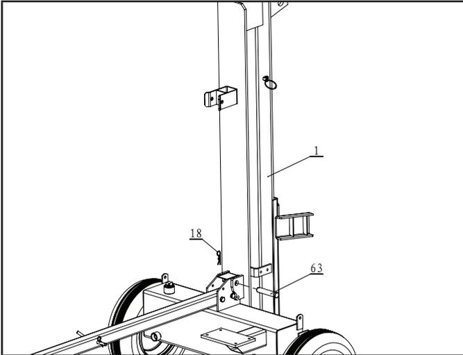
4. Block the wheels to prevent the frame from rolling.
