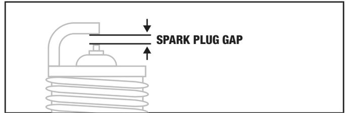
5. Refer to the spark plug section on the *Specifications* page when replacing the plug.
