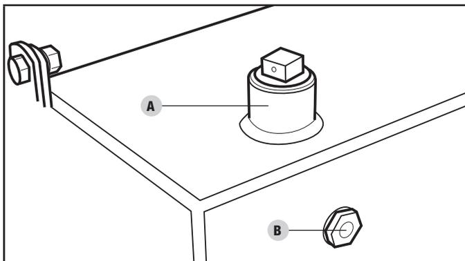
8. Unscrew and remove the tank fill plug, on top of the tank. Using a funnel add approximately 4 gal. (15.1 L) of hydraulic oil to the tank. Wipe up any spilled oil. (A)
