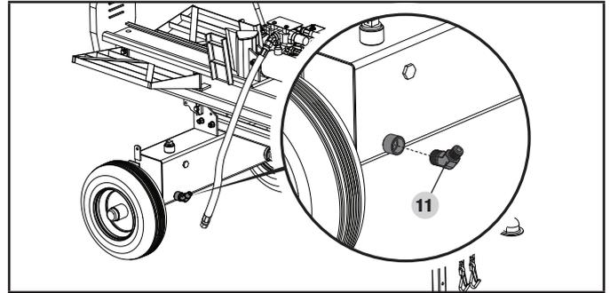
7. Place an o-ring into tank inlet connector installed in the previous step. Make sure the o-ring is properly placed in the inner groove. Connect the end of hose (19) to the tank inlet connector. Securely tighten the end with a 27mm wrench (Torque: 52 lbf-ft (70.5 Nm) to 66 lbf-ft (89.5 Nm)).
