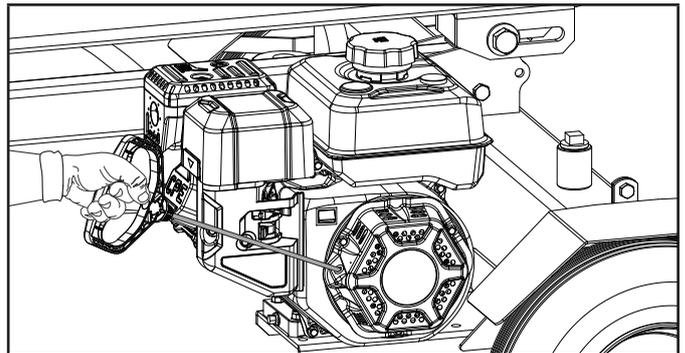
5. As engine warms up, move the choke lever to the "RUN" position.
