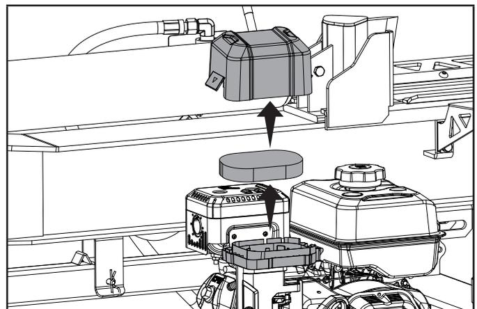
3. Wash in liquid detergent and water. Squeeze thoroughly dry in a clean cloth.
