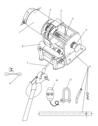
Motor (1): .7 HP 12V DC motor provides power to the planetary gear mechanism. Planetary Gear System (2): The reduction gears convert the winch motor power into extreme pulling forces. This system allows high torque while maintaining compact size and light weight.
