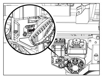
If the engine starts but does not run make certain that the log splitter is on a flat, level surface. The engine is equipped with a low oil sensor that will prevent the engine from running when the oil level falls below a critical threshold.
