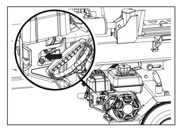
3. Move the fuel valve to the "ON" position.
