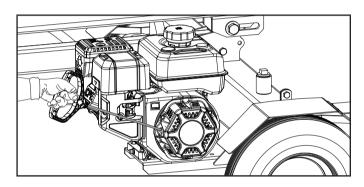
As engine warms up, move the choke lever to the "RUN" position.
