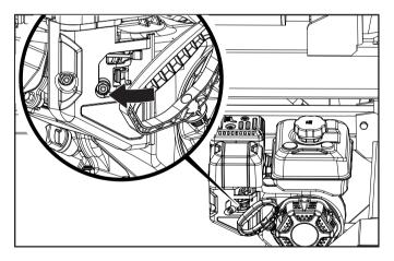
2. Let the engine run until fuel starvation has stopped the engine. This usually takes few minutes.
