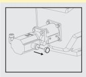
Hydraulic pump may contain residual oil from testing procedures during production.
