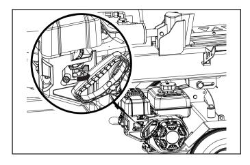
4. Pull the starter cord until resistance is felt and then pull rapidly.
