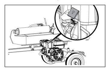
2. Remove both air filter cover and air filter element.
