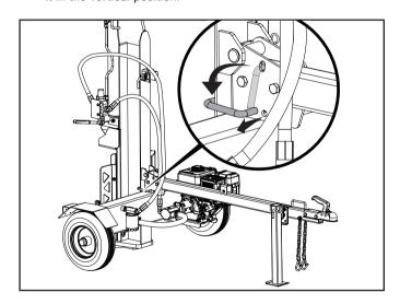
4. To change from vertical to horizontal orientation, reverse the steps. The beam will automatically lock into the auto-lock on the tow bar when lowered into position.
