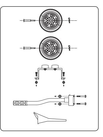
Your generator requires some assembly. This unit ships from our factory without oil and fuel. It must be properly serviced with fuel and oil before operation.
