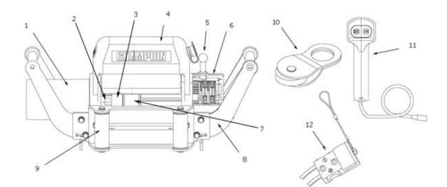
**Motor (1)**: 3.6 HP 12V DC motor provides power to the planetary gear mechanism.
