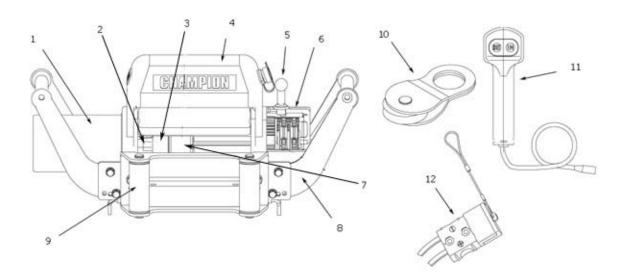
**Motor (1)**: 3.6 HP 12V DC motor provides power to the planetary gear mechanism.
