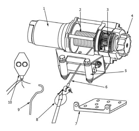
**(1) Motor**: 1.2 HP (0.89KW) 12V DC motor provides power to the planetary gear mechanism.
