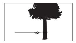
Your winch is equipped with a roller fairlead to help guide the cable/rope and to reduce binding on short side pulls. Do not winch from an acute angle as the cable/rope will pile up on one side of the drum causing damage to cable/rope and the winch.
