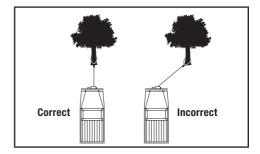
Short pulls from an angle can be used to straighten the vehicle. Long pulls should be done with the cable/rope at a 90° angle to the winch/vehicle. When pulling a heavy load, place a blanket or jacket over the cable/rope 5-6′  $(1.5-1.8\ m)$  from the hook. In the event of a broken cable/rope it will dampen the snap back.
