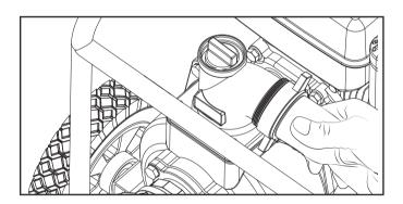
5. Slide the hose clamp in place about midway on the outlet hose adapter as shown. Tighten to  $7.4\pm1.5$  lbf-ft ( $10\pm2$  Nm) with a 10mm wrench. The hose clamp should be placed behind the outlet adapter barbs on the smooth part of the adapter.
