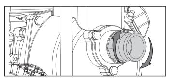
15. Attach the cam lock coupler to the fitting.
