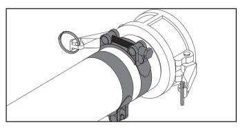
9. Rotate and align the clamp bolts so you have clearance for the cam levers to lock in place later.
