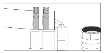
6. Slide the clamps back and start to assemble the green hose to cam lock coupler.
