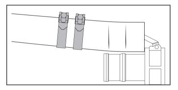
7. Insert the cam lock coupler in the green rigid suction hose until properly seated.
