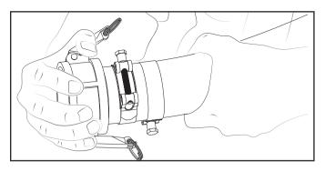
13. Wrap the green inlet clockwise with the Teflon<sup>®</sup> tape provided with 4 complete wraps.
