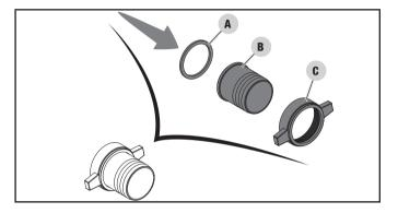
2. Thread the assembled connector to the outlet fitting (top of pump).
