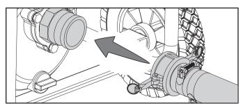
16. Lock in place with the cam levers.
