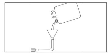
Pour the antifreeze into the funnel, then pull on the engine recoil starter to create suction in the pump housing. Pull the recoil several times until antifreeze comes out of the pump outlet. DO NOT START THE ENGINE WHEN DOING THIS. Only pull the recoil cord if the fuel valve and engine switch are in the OFF position.
