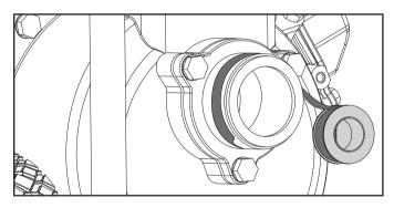
14. Thread the fitting over the tape and hand tighten. Use either 14" Channellock® or a pipe wrench with 2.5" (63.5mm) opening min, hand tight then 1 1/2 turn past full tight. This is critical to make sure the fitting is tight so you do not have air leaks.
