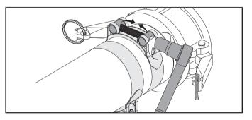
11. Once tightened, visually confirm the hose is raised on the ribs. This indicates you have it tight.
