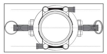
10. Tighten each clamp to  $11.1\pm1.5$  lbf-ft ( $15\pm2$  Nm) with a 10mm socket and 3/8" drive ratchet until the clamp completely tightens. If you do not have a torque wrench, hand tight then  $\frac{1}{4}$  turn past full tight. This will need to be as tight as you can make them.
