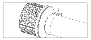
21. Tighten the clamp to  $7.4\pm1.5$  lbf-ft ( $10\pm2$  Nm) with a 10mm wrench. If you do not have a torque wrench, hand tight then  $\frac{1}{4}$  turn past full tight.
