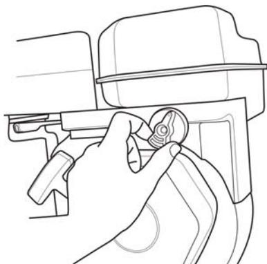
4. Move the choke lever (Item A) to the "Choke" position (to the left).
