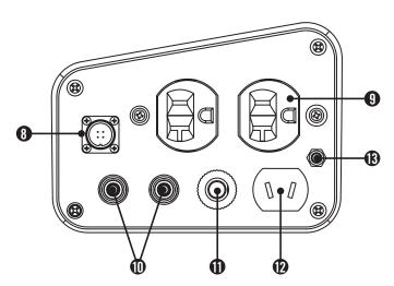
\* These outlets are used for connecting two Champion model 73536i generators for parallel operation.
