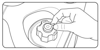
4. Turn the fuel valve to the "On" position.
