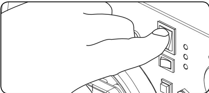
7. **ELECTRIC START:** Press and hold the ignition switch to the "START" position. Release as the engine begins to roll over. If the engine fails to start
