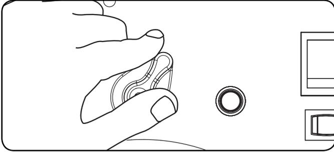
4. Turn the battery switch to the "On" position.
