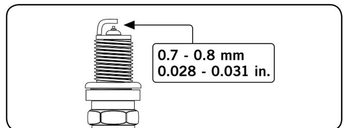
5. Refer to the spark plug recommendation chart when replacing the plug.
