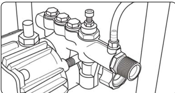
Place the filter end of the detergent hose into pressure washer detergent (not included).
