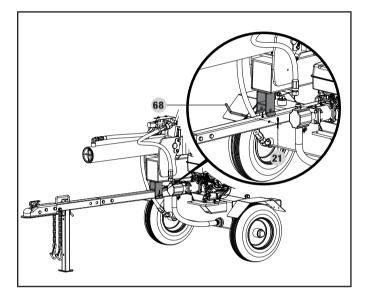
3. Insert pin and "R" clip in the rear locking hole (at base of tow beam).
