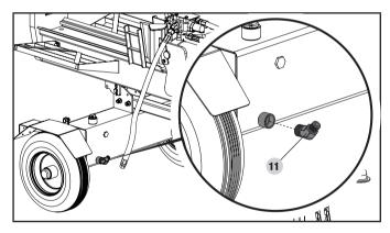
Place an o-ring into tank inlet connector installed in the previous step. Make sure the o-ring is properly placed in the inner groove. Connect the end of hose (17) to the tank inlet connector. Securely tighten the end with a 27mm wrench (Torque to 44 - 52 ft lbs.).
