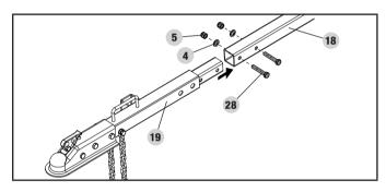
2. Attach the tow bar to the bracket on top of the hydraulic oil tank with two M12  $\times$  85 bolts (64) and M12 lock nuts (5) and washers (4).
