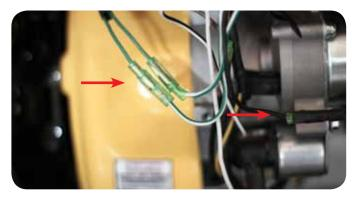
2) Locate the Black wire with a soft Black rubber covering on the connection point. This is for the Ignition system and is a grounding function wire. Unplug this connection.
