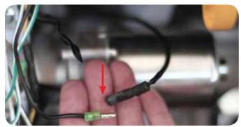
3) Next you will locate a single black harness that has two Green wires inside the loom. Each green wire will have either a black or white stripe on the green insulation covering the wire. Unplug either green wire. Only one of them is necessary.
