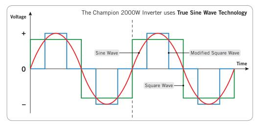
wave and modified square wave inverters. The waveform of these types of inverters is a rough, stepped, digital approximation of a TSW. See the graph to the left.
