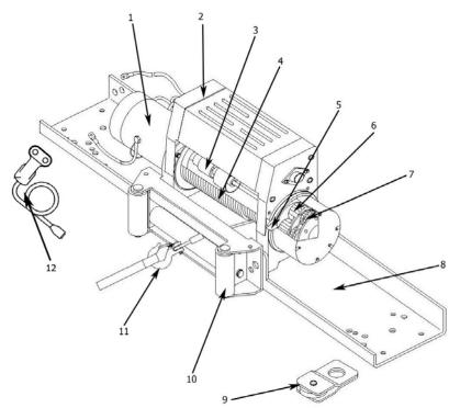
(1) Motor: 3.6 HP 12V DC motor provides power to the planetary gear mechanism.
