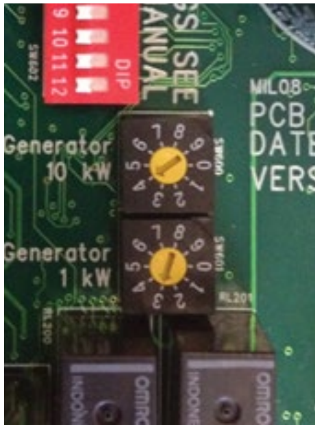
Figure 6 – Generator Power Rotary Switches
