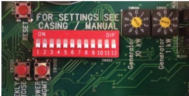
Figure 7 – DIP Switches on the Control Board
