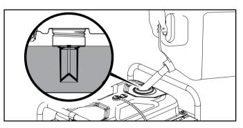
3. The approximate fuel level is shown on the fuel gauge on top of the fuel tank.
