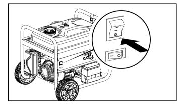
4. *If generator was started electrically*, press the battery switch to the "OFF" position.
