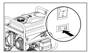
2. Press and hold the ignition switch to the "START" position. Release as the engine begins to start. If the engine fails to start within five seconds, release the switch and wait at least ten seconds before attempting to start the engine again.
