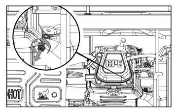
5d. When gasoline stops flowing from the carburetor, replace and tighten the carburetor drain bolt and be sure to properly dispose of the drained gasoline according to local regulations or guidelines.
