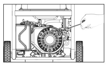
6. Do not over-choke. As soon as engine starts, move the choke to the "RUN" position over a 2-5 second duration.
