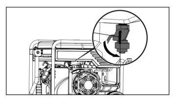
4. Pull the choke to the "CHOKE" position.
