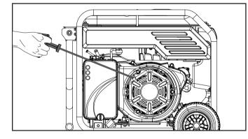
4. Once engine starts, push choke button to the "RUN" position.
