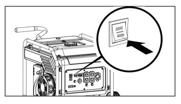
2. Once engine starts, push choke button to the "RUN" position.
