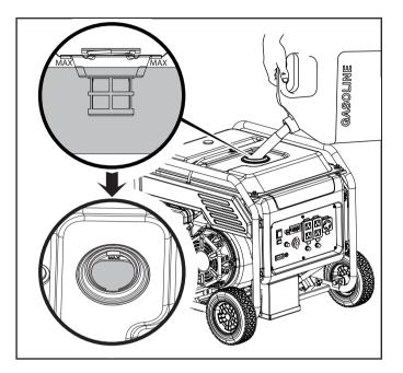
3. Fuel gauge on top of tank will read "F" when full of gasoline and "E" when tank is empty and needs to be refilled.
