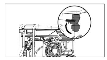
**Important:** Always ensure that the fuel valve and the engine switch are in the "OFF" position when the generator will not be used for an extended period of time.
