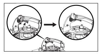
To release, move the cruise control lever back to the original low position.
