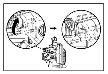
3. Slowly press the primer bulb 7-14 times or until fuel is visible and flows freely into the clear tank return line.
