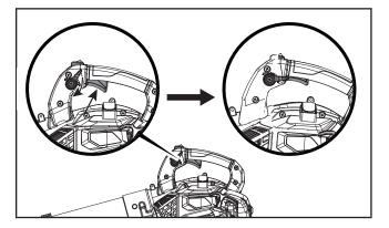
Holding the unit firmly, pull starter grip until engine starts. Use short pulls and do not allow the rope to snap back. Do not pull more than 6 times.
