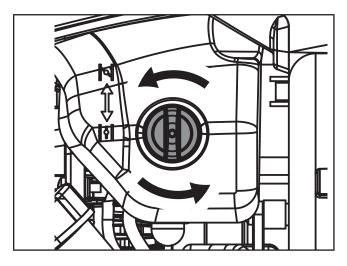
3. Inspect and replace or clean the air filter. To reassemble make sure the filter fits in the cavity and reinstall the filter as shown. Fasten the air filter cover by turning the fasteners clockwise.
