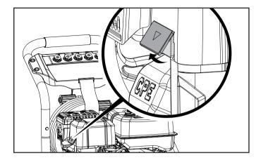
2. Remove both air filter cover and air filter element.
