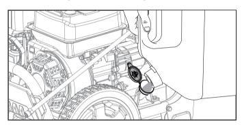
Insert the detergent suction hose (end with the filter) through the detergent tank cap until it goes all the way to the bottom of the detergent tank.
