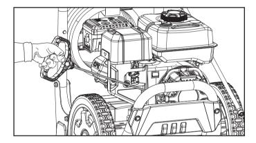
5. As engine warms up, move the choke lever to "RUN".
