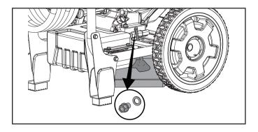
3. Replace the oil drain bolt.
