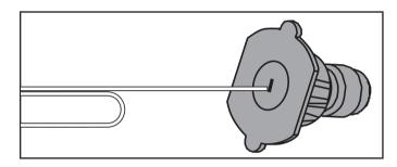
To prevent accidental starting, remove and ground spark plug wire before performing any service.
