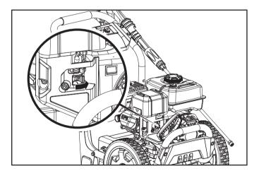
3. Move the choke lever to the "CHOKE" position.
