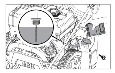
4. Check engine oil level at every use and add as needed.
