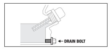
2. Allow the oil to drain completely into an appropriate container.
