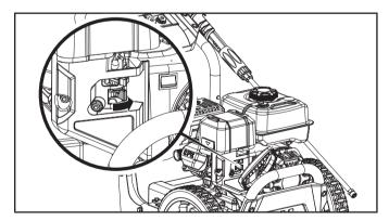
3. Move the choke lever to the "CHOKE" position.
