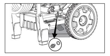
3. Replace the oil drain bolt.
