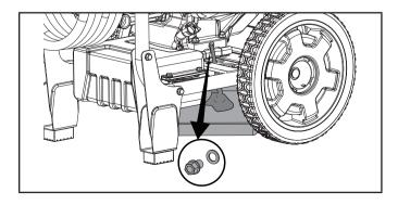
3. Replace the oil drain bolt.
