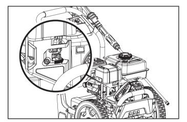
3. Move the choke lever to the "CHOKE" position.
