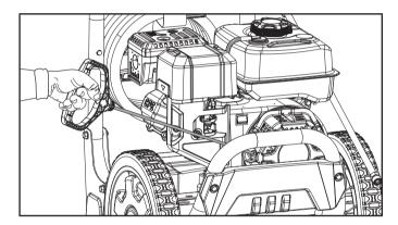
5. As engine warms up, move the choke lever to "RUN".
