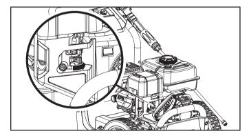
3. Move the choke lever to the "CHOKE" position.
