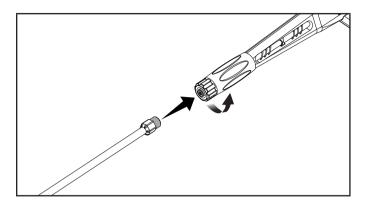
3. Connect the end of the high pressure hose to the gun inlet. Tighten connection clockwise. Do not overtighten.
