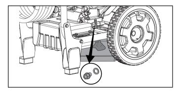
3. Replace the oil drain bolt.
