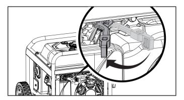
5. Press engine switch to "ON" position.
