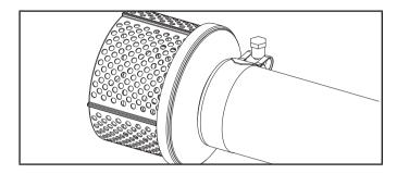
8. Tighten the clamp to 7.4±1.5 lbf-ft (10±2 Nm) with a 10mm wrench. If you do not have a torque wrench, hand tight then ¼ turn past full tight.
