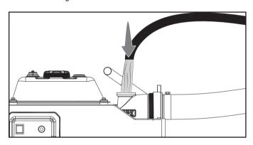
As the engine starts up, this will start the draw of liquid into the pump. Located within the pump assembly is the oneway valve. As you prime the pump housing this one-way flap valve shuts off the opening to the suction hose. The priming process is only required when the pump housing is not full of water.
