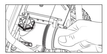
5. Slide the hose clamp in place about midway on the outlet hose adapter as shown. Tighten to 7.4±1.5 lbf-ft (10±2 Nm) with a 10mm wrench. The hose clamp should be placed behind the outlet adapter barbs on the smooth part of the adapter.
