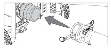
3. Lock in place with the cam levers.
