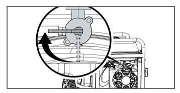
2. Let the engine run until fuel starvation has stopped the engine. This usually takes a few minutes.
