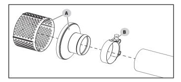
6. Place the clamp marked 54-57 on the other end of the green hose. Attach the strainer to the green suction hose.
