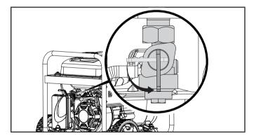
4. Push the engine switch to the "ON" position.
