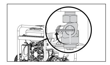
**Important:** Always ensure that the fuel valve and the engine switch are in the "OFF" position when the generator is not in use.
