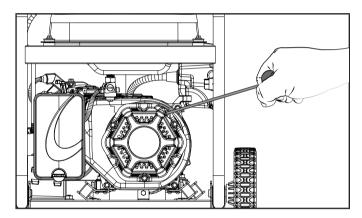
7. As soon as engine starts, move the choke to the "RUN" position over a 2-5 second duration.
