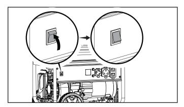
5. Move the choke to the "CHOKE" position. Note: for restarting a warm engine, move the choke to 75% of the CHOKE position.
