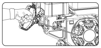
7. As engine warms up, move the choke lever to "Run."(D)
