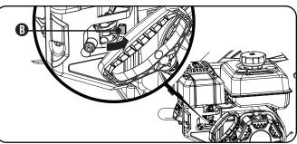
5. Move the choke lever to the "Choke" position. (C)
