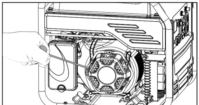
7. As engine warms up, push the choke knob in to the "RUN" position.
