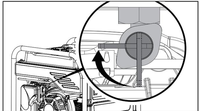
4. Let the engine run until fuel starvation has stopped the engine. This usually takes a few minutes.
