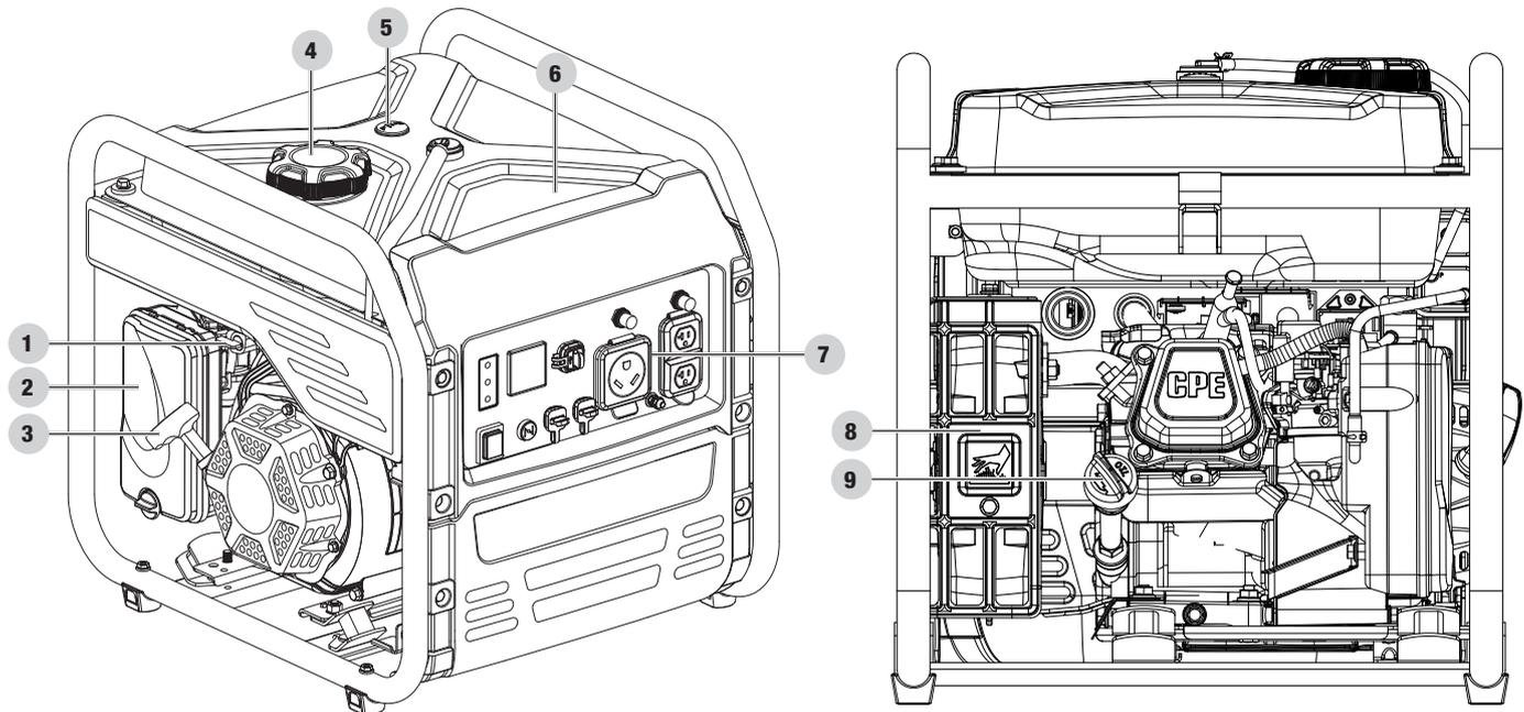
1. **Fuel Valve** – Used to turn fuel supply on and off to engine.
