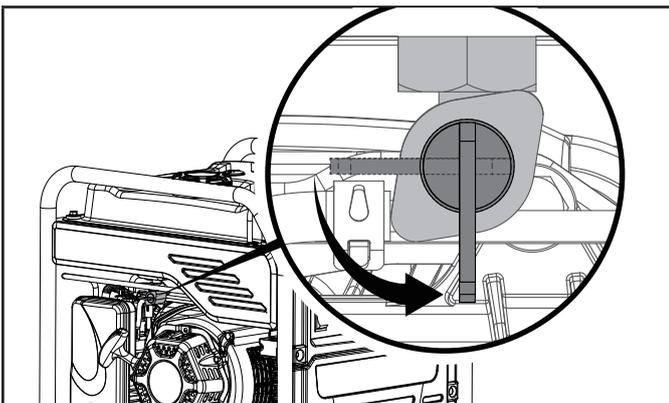
4. Turn the engine switch to the "ON" position.
