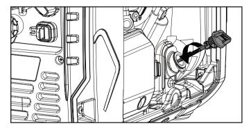
4. Tilt the generator on its side and allow the oil to drain completely.
