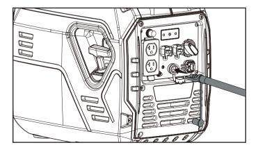
7. Check all connections for leaks by wetting the fittings with a solution of soap and water. Bubbles which appear or bubbles which grow indicate that a leak exists. If a leak exists at a fitting then turn off the valve on the cylinder and tighten the fitting. Turn the valve back on and recheck the fitting with the soap and water solution. If the leak continues or if the leak is not at a fitting then do not use the generator and contact customer service.
