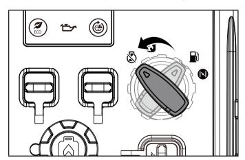
**Important:** Always ensure that the dial and fuel vent on the fuel cap are in the "OFF" position when the generator is not in use.
