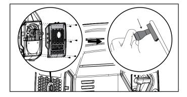
6. Replace the spark arrestor if it is damaged.
