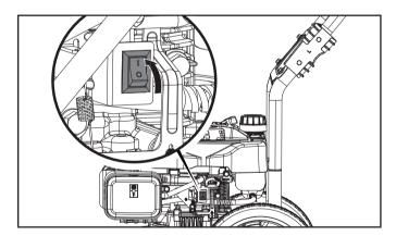
3. Move the choke lever to the "CHOKE" position.
