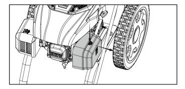
2. Remove both air filter cover and air filter element.
