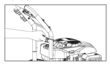
6. As engine warms up, move the choke lever to "RUN".
