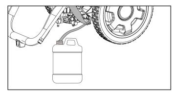
Install the quick connect detergent nozzle (black) in the spray wand. Detergent will only be drawn through the pump when the black detergent nozzle is attached to the end of the wand. Be sure water supply is on. Start the engine. Pull the trigger gun to spray the detergent solution.
