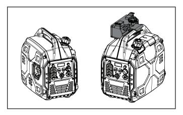
4. Place the bracket around the handle and tighten the fastening dial by turning clockwise until snug. Do not over tighten. You may need to loosen the fastening dial to get it around the handle before tightening.
