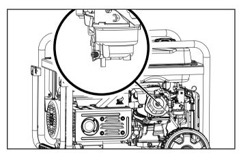
5d. When gasoline stops flowing from the carburetor, replace and tighten the carburetor drain screw and be sure to properly dispose of the drained gasoline according to local regulations or guidelines.
