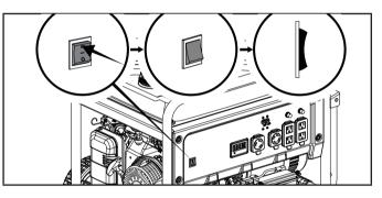
3. Do not over-choke. As soon as engine starts, move the choke to the "RUN" position over a 2-5 second duration.
