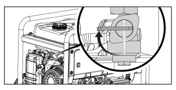
**Important:** Always ensure that the fuel valve and the ignition switch are in the "OFF" position when the generator is not in use.
