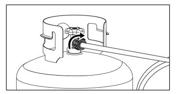
4. Reference your generator's instruction manual to correctly attach the LPG hose and regulator assembly to your generator.
