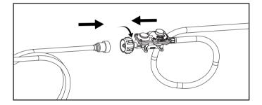
3. Attach the female end of the extension hose to the LPG tank by turning the connector clockwise to tighten.
