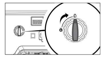
**Important:** Always ensure that the fuel dial is in the "OFF" position when the generator is not in use.
