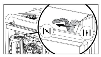
Press and hold the ignition switch to the "START" position. Release as the engine begins to start. If the engine fails to start within five seconds, release the switch and wait at least ten seconds before attempting to start the engine again.
