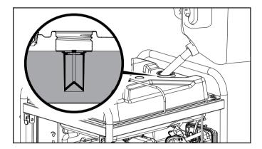
The approximate fuel level is shown on the fuel gauge on top of the fuel tank.
