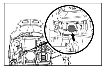
4. Set the cruise control lever to the half throttle position.
