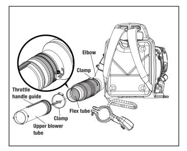
3. Loosen wing nut completely on throttle handle clamp. Align notches in throttle handle clamp with guide on the upper blower tube and slide on as shown. When the throttle handle is at the desired length, tighten the wing nut fully to secure.
