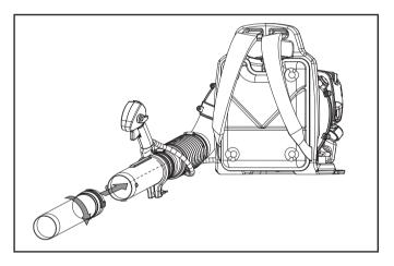
5. Assemble middle blower tube to lower blower tube by aligning the arrow of the peg of tube with the arrow of the locking groove of tube. Slide the peg into the locking groove and rotate clockwise to lock in place.
