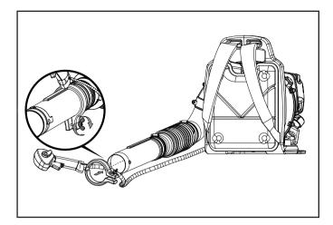
4. Assemble upper blower tube to middle blower tube by aligning the arrow of the peg of tube with the arrow of the locking groove of tube. Slide the peg into the locking groove and rotate clockwise to lock in place.
