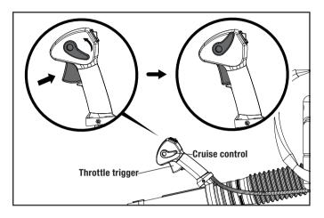
To release, move the cruise control lever back to the original low position.
