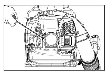
6. Move choke knob to the RUN position and pull recoil starter handle until engine starts. Do not pull more than 6 times.
