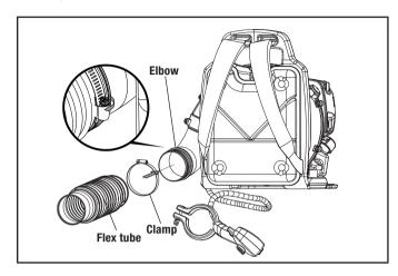
2. Install flex tube to upper blower tube (with the throttle handle guide). Tighten the clamp fully.
