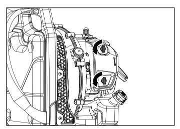
Inspect and replace or clean the air filter. To reassemble make sure the filter fits in the cavity and reinstall the filter as shown. Fasten the air filter cover by turning the fasteners clockwise.
