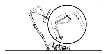
6. Using your right hand, pull the starter cord slowly until resistance is felt and then pull rapidly.
