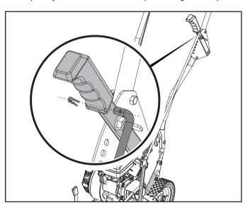
2. Insert the other end of the control rod through the hole on the blade adjust arm and secure it in place using the R-clip.
