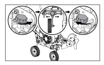
Adjust the front wheel height by pulling the lever outward to disengage it from the locking tab and moving the lever downward until the desired height is met then place the lever back onto the locking tab at this position.
