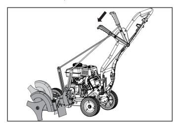
Once done with the edging task, again pull the blade depth adjust handle outward (to the left) to disengage the locking tab then move the lever upward locking into the to the top storage position.
