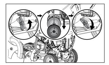
Start the engine (see the Starting the Engine section), set your edging depth (see the Adjust the Edging Depth section) and start edging along the curb. 100731 - LAWN EDGER MAINTENANCE
