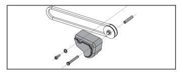
5. Using a 8 mm wrench or socket remove the two screws from the front pulley guard and remove the guard.
