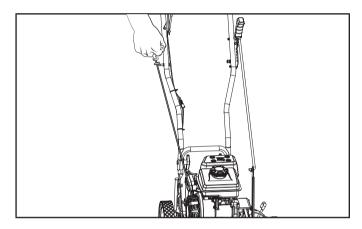
7. As the engine warms up, move the choke lever to the "RUN" position.
