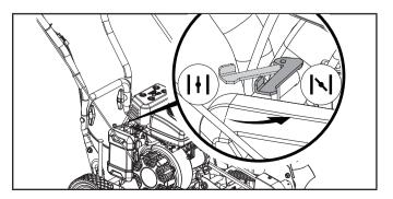
5. Using your left hand, pull the control handle to the upper handle to engage the starting mechanism.
