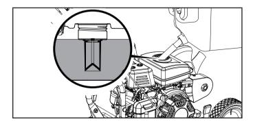
3. Screw on the gasoline cap and wipe away any spilled fuel.
