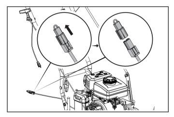
2. Connect the engine ground wire to the handle ground wire.
