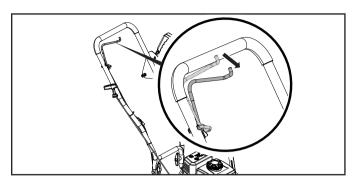
2. Rotate the fuel valve to the "OFF" position.
