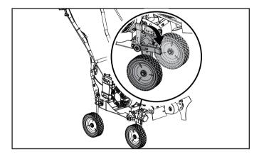
Loosen the rear wheel locking knob by rotating it counterclockwise then adjust the wheel downward to match the height of the front wheel. Rotate the rear wheel locking handle clockwise and tighten securely.
