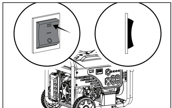
2. Turn the battery switch to the "ON" position.
