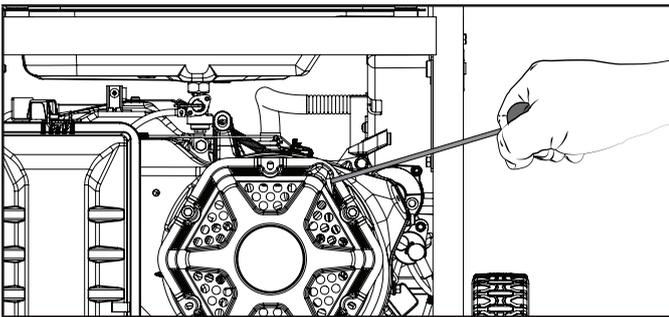
5. Do not over-choke. As soon as engine starts, move the choke lever to the “RUN” position over a 2-5 second duration.
