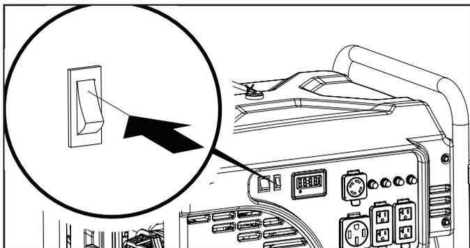
2. Push the ignition switch to the "ON" position.
