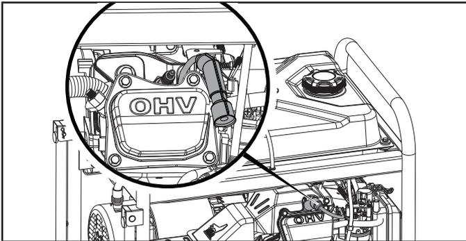
3. Inspect the electrode on the plug. It must be clean and not worn to produce the spark required for ignition.
