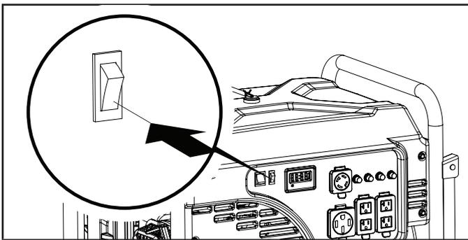
3. Push and hold the wireless set button found on the side of the control panel for approximately three seconds until the red light turns on.
