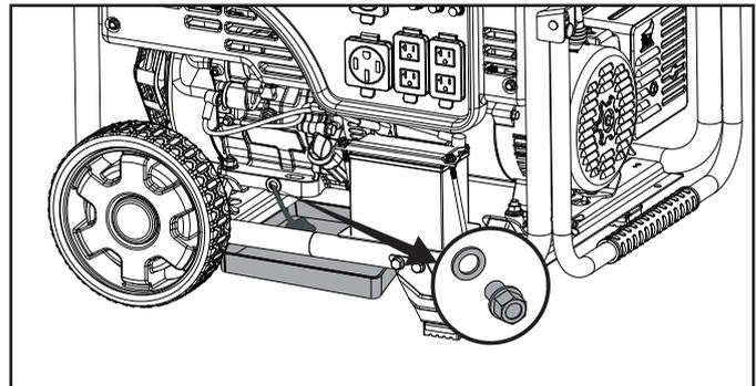
3. Replace the oil drain bolt.
