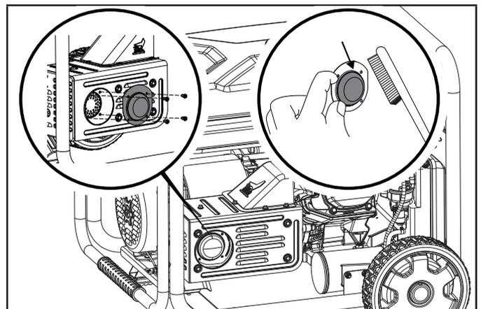
5. Replace the spark arrestor if it is damaged.
