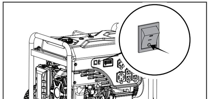
4. *If generator was started electrically*, press the battery switch to the “OFF” position.
