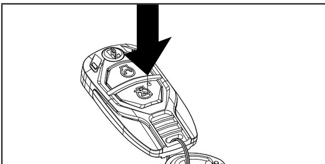
5. Push and release the START button on the remote key fob. The red light blinks once to program the remote.
