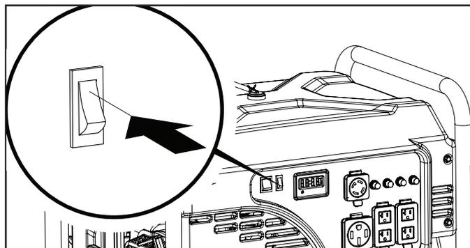
2. Press and hold the ignition switch to the "START" position. Release as the engine begins to start. If the engine fails to start within five seconds, release the switch and wait at least ten seconds before attempting to start the engine again.
