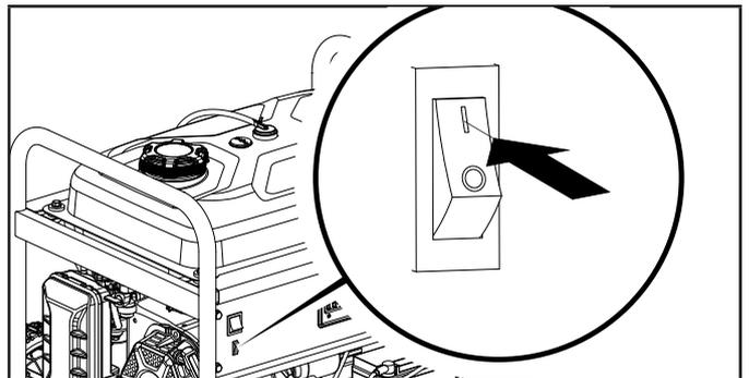
2. Press and hold the ignition switch to the "START" position. Release as the engine begins to start. If the engine fails to start within five seconds, release the switch and wait at least ten seconds before attempting to start the engine again.
