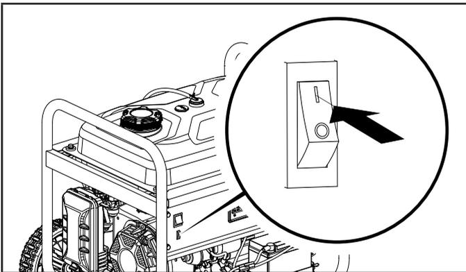
2. Push the ignition switch to the "ON" position.
