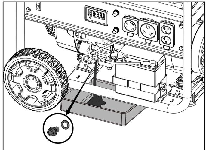
3. Replace the oil drain bolt.
