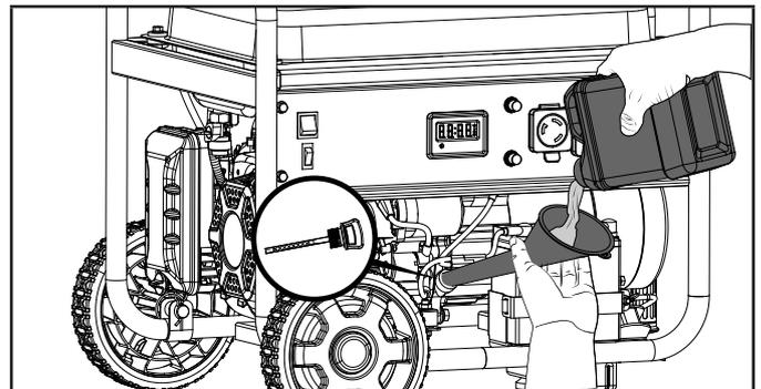
4. Check engine oil level at every use and add as needed.
