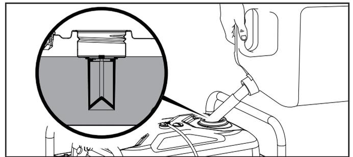
3. The approximate fuel level is shown on the fuel gauge on top of the fuel tank.
