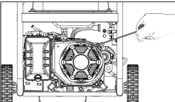
5. Do not over-choke. As soon as engine starts, move the choke lever to the "RUN" position over a 2-5 second duration.
