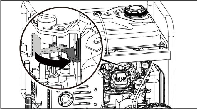
3. Push the ignition switch to the "ON" position.
