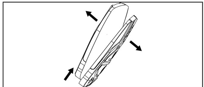
5. Carefully remove the circuit board to locate and replace the CR2016 battery.
