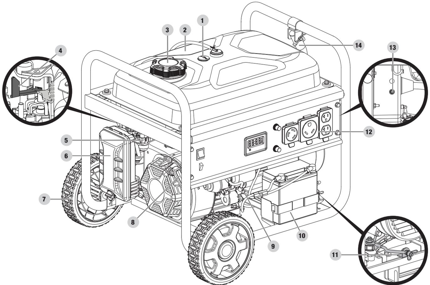
1. **Fuel Gauge** – Indicates the amount of gasoline in the fuel tank.
