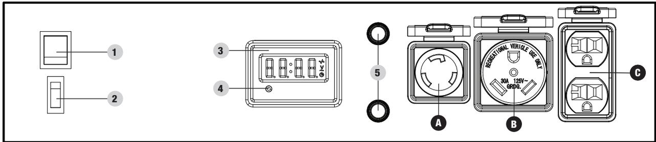
1. **Ignition Switch** – Used to START or STOP the generator.
