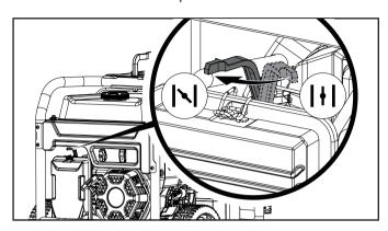
Press and hold the ignition switch to the "START" position. Release as the engine begins to start. If the engine fails to start within five seconds, release the switch and wait at least ten seconds before attempting to start the engine again.
