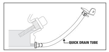
Point the hose into a drain pan and allow the oil to drain completely.
