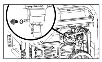
5d. When gasoline stops flowing from the carburetor, replace and tighten the carburetor drain bolt and be sure to properly dispose of the drained gasoline according to local regulations or guidelines.
