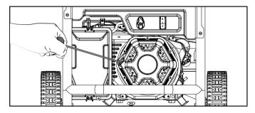
4. Do not over-choke. As soon as engine starts, move the choke lever to the "RUN" position over a 2-5 second duration.
