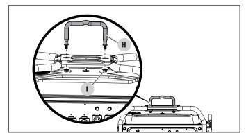
2. Tighten bolts securely to a torque of 17-22 ft-lbs.
