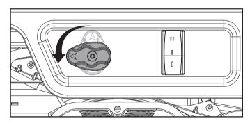
**Important:** Always ensure that the fuel valve and the ignition switch are in the "OFF" position when the generator is not in use.
